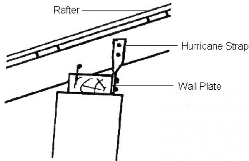
**Hurricane strap holding down rafter to wall plate.**
